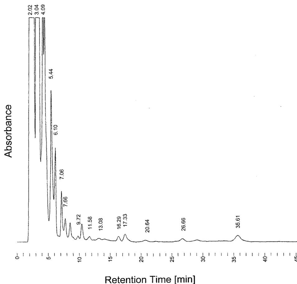
Figure 1. An HPLC profile of products after two-hour trial. All samples were analyzed by YMC hydrosphere C18 column ( $150 \times 4.6$  mm  $\varnothing$ ). The mobile phase consists of 50 mM K-phosphate buffer pH = 2.5 and 7.2 mM Na-hexasulfonate. The flow rate of the mobile phase was  $1.0 \text{ mL min}^{-1}$ . Profile intensity was absorbance at 195 nm.
